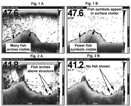
Figures 1A and 2A (left) show Sonar Page in normal chart mode. Figures 1B and 2B (right) show the same underwater scene with Fish I.D. turned on. Note how arches are replaced with symbols.
